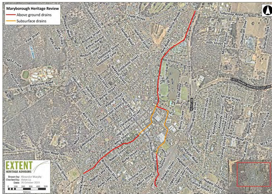
Figure 2. Aerial map showing both above ground and subsurface portions of the Main Drain, Maryborough.
