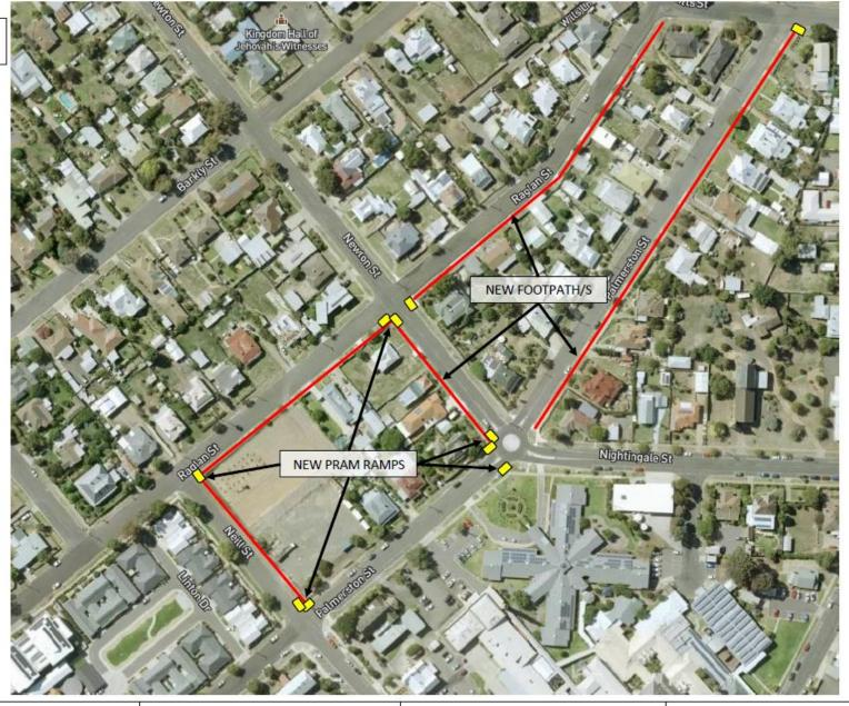
PIC REF: 046 - 050 **IMPLEMENT NEW PED CROSSING & PRAM** RAMPS TO PROTECT PEDS FROM VEHILCES **ENTERING & EXITING CAR PARK** 101-108 PED CROSSING CSD CHECKS NEEDED - IF NOT MET CONSIDER CHANGES TO PARKING IMPLEMENT NEW PED CROSSINGS & WIDEN PED REFUGES
