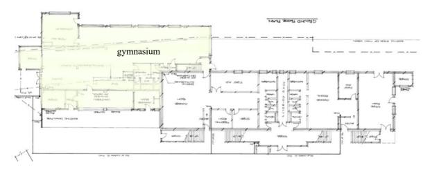
In 1977 plans were prepared to upgrade the existing lower ground level clubrooms shown on the left and construct an addition to the Grandstand as shown above. The new Club Rooms extended to the rear of the grandstand where access was created to a large gymnasium and also stairs to access the upper level of the new building.
