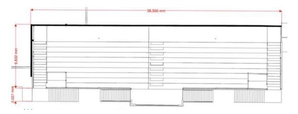
Plan of raked seating area in the Maryborough Grandstand with a size of 38,566mm by 9832mm with external brick and concrete stairways of 2,027mm width.
