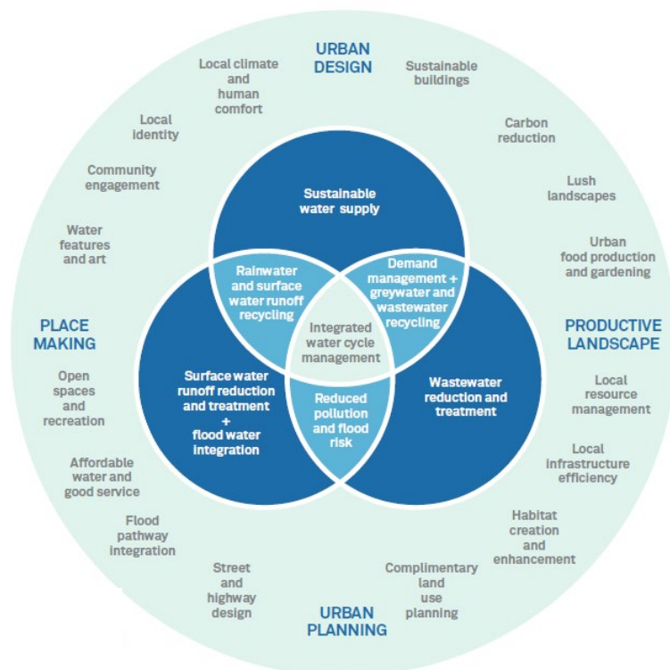
Figure 1.1: Integrated water management diagram showing the interaction of the three ‘types’ of water within a context of urban form and landscapes.
