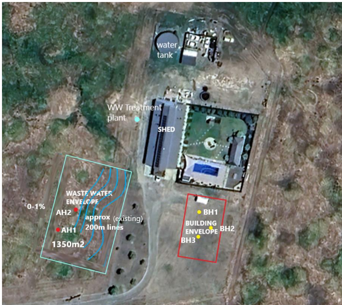
Fig 5 Location of proposed new dwelling (red), waste water envelope showing location of existing 200m irrigation lines and additional area (total 1350m 2 ) to allow installation of an extra 200m irrigation lines. Location of auger holes (AH) and geotechnical boreholes (BH) slope and site features.
