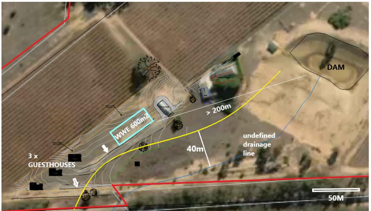
Figure 7 Map showing southern part of the subject property with area nominated for group accommodation with WWEs (600m 2 ) available for secondary treatment with a 40m setback.
