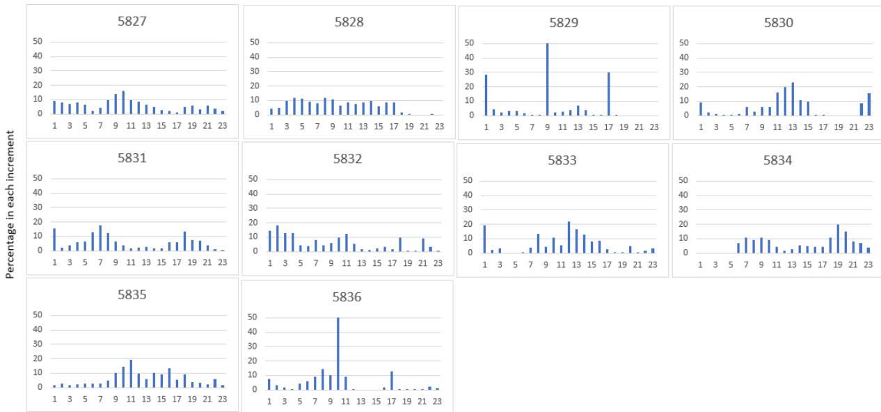
FIGURE 2-6 AREAL TEMPORAL PATTERNS FOR SOUTHERN SLOPES (MAINLAND) FOR 72 HOURS, AND CATCHMENT AREA OF 1000 KM 2
