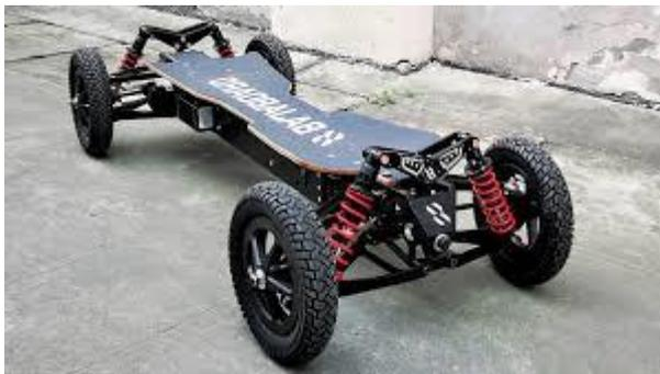
*Off road electric powered skateboard (Source: bajaboard.com.au)*
