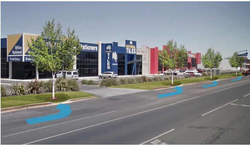
Stormwater drainage to water street trees in new developments
