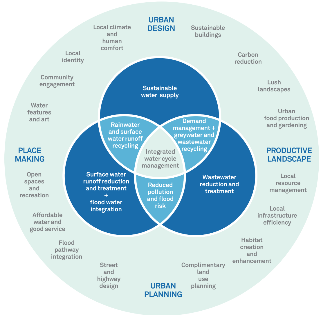
Integrated water management diagram showing the interaction of the three 'types' of water within a context of urban form and landscapes.
